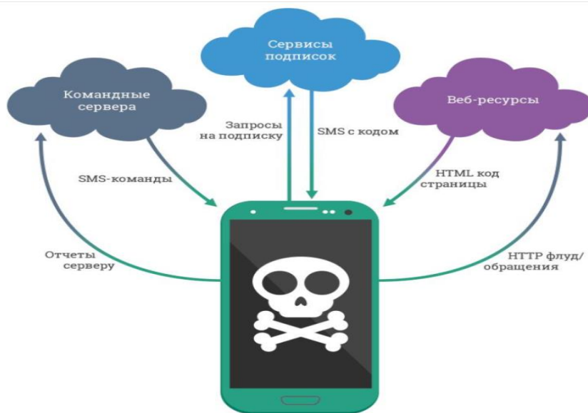
Figure 1 – Work algorithm Trojan-SMS programs for mobile devices
